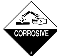
Risk of Burns from Battery Acids
